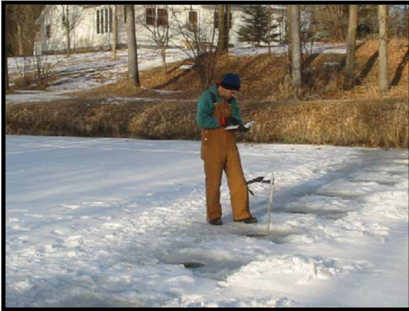
Measuring flow beneath ice
