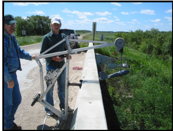
Measuring flow with bridge crane
