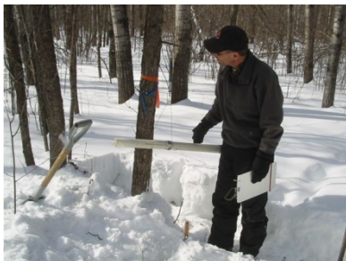
Establish base weight of empty sampling tube
