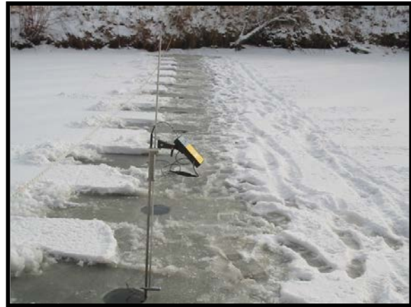
Measuring flow beneath ice
