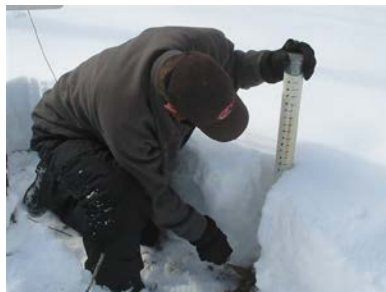
Obtaining snow depth and core sample
